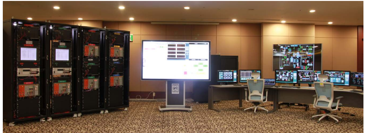
Prototype of Digital Protection System and Nuclear Simulator
